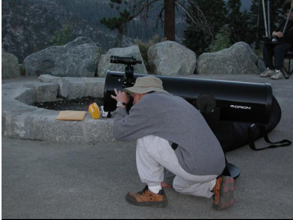
Craig Harrison aligns the finder on his 10-inch dobsonian using the peak of Half Dome.
