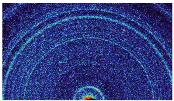
The first x-ray crystallography view of Martian soil. Obtained by the Chemistry and Mineralogy (CheMin) experiment on NASA's Curiosity rover, these data reveal crystalline feldspar, pyroxenes and olivine mixed with some amorphous (non-crystalline) material. The soil sample is similar to volcanic soils in Hawaii. [more]
